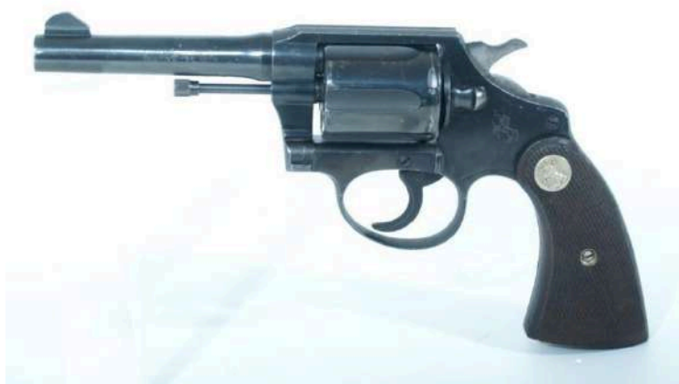
Revolver Colt Police Positive calibre .38 S&W.
